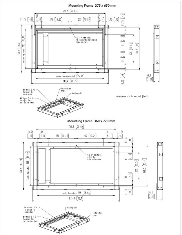
Garland Induction Built-in Unit RTCSmp Module-Line "Two Cooking Zones" Induction Green Heat
